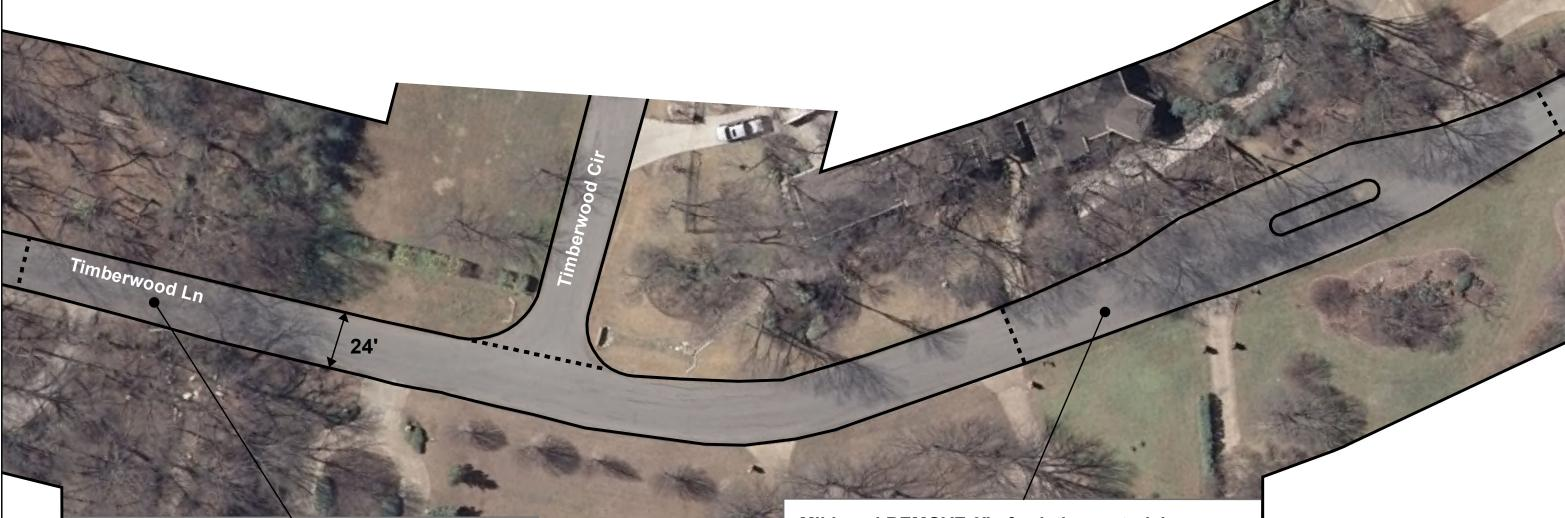
MILL and RECYCLE existing asphalt and base to 6" depth. INSTALL cement slurry at a rate of 28 lbs per S.Y. LEVEL & COMPACT to 95% density while applying moisture. INSTALL Prime Coat and 92.2 tons of 1" Type D HMAC leveling course. A = 1,130 S.Y. NO tack Coat Required. (Reinforced fiberglass grid with Ultrafuse coat to be installed by others.) INSTALL 92.2 tons of 1 1/2" Type D HMAC surface course. A = 1,130 S.Y.
